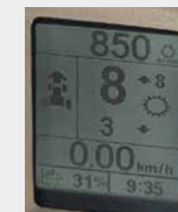
PUMA MULTICONTROLLER MODELS: THE RANGE AND GEAR SELECTIONS ARE CLEARLY SHOWN ON THE A-PILLAR DISPLAY
